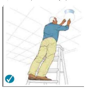
6.8.12 When using stepladders, avoid work that imposes a side loading, such as sideon drilling through solid materials (e.g. bricks or concrete), by having the steps facing the work activity. Where side-on loadings cannot be avoided you should prevent the steps from tipping over, for example by tying the steps to a suitable point, or you should use a more suitable type of access equipment.
